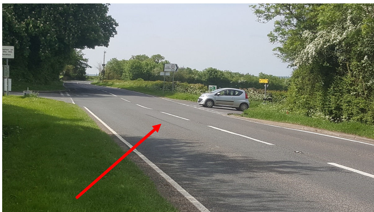
Figure 10 - skid mark on A426; evidence of a near miss or a damage only collision
