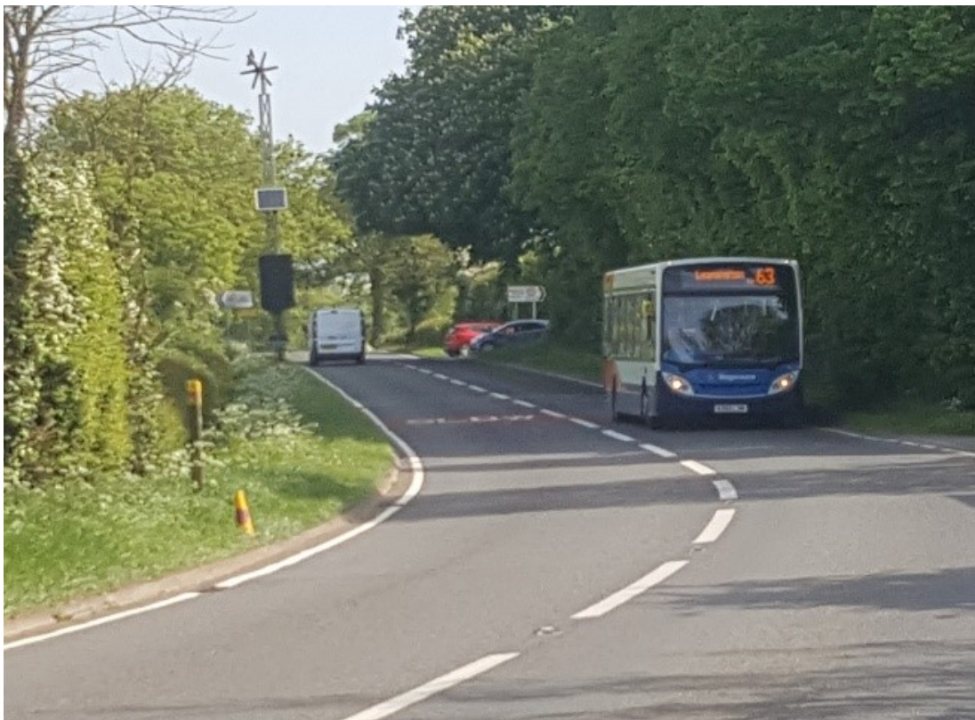
Figure 37 - offside cross-roads warning sign masked by bus
