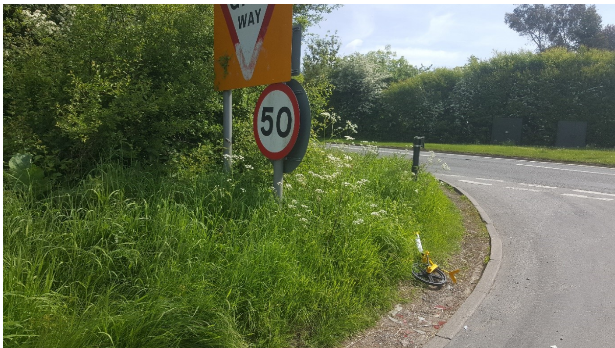
Figure 31 - speed limit sign should not be co-located with give way sign
